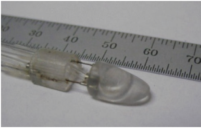
Fig. 40.4 The dual-chamber body of the HeartLander robot allows for it to move along the heart via an inchworm-like motion actuated through a suction mechanism. The small design allows for insertion via a small incision below the sternum and applications in minimally invasive heart surgery. (Courtesy of Cameron Riviere, from Tortora et al. [12])
