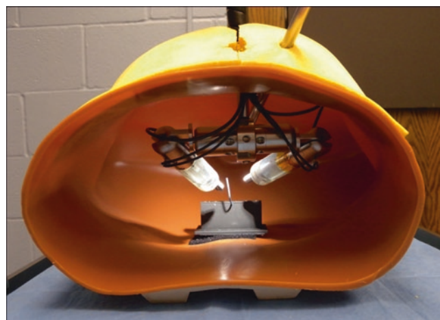
Fig. 39.1 Robot platform is inserted into the abdomen in this model. When expanded, it will have two working arms and a camera, each with its own range of motion
