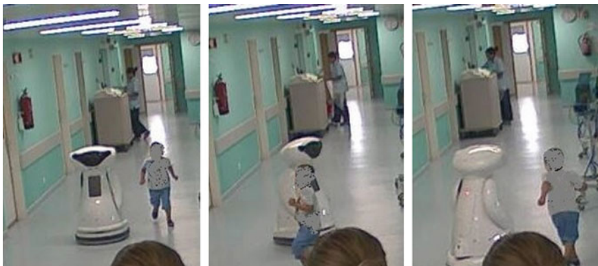
Fig. 2.8 The MOnarCH robot using a “dancing” movement for expressivity (the sequence evolves from left to right)
