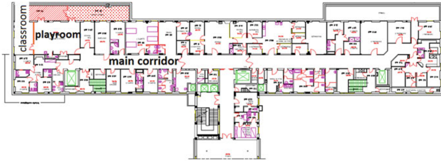
Fig. 2.4 The blueprint of the Pediatrics ward; the areas marked “classroom”, “playroom”, and “main corridor” can be used by the robot
