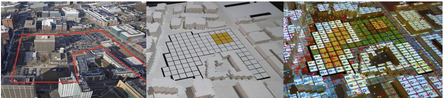
Fig. 2. Abstraction process from the actual urban area into an interactive LEGO model which interfaces with mathematical models and simulations.
