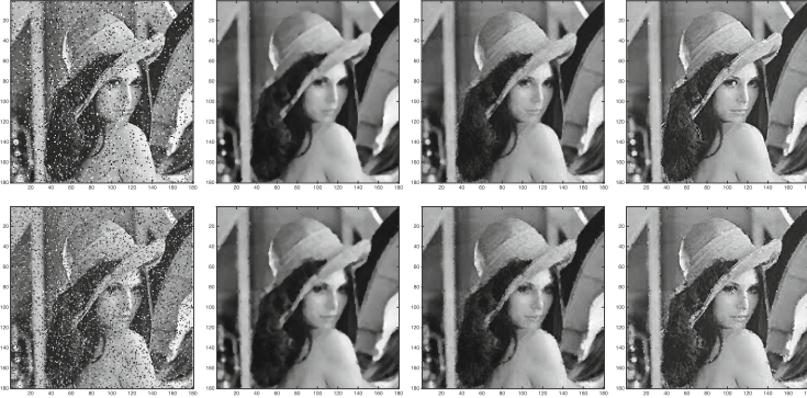
Fig. 4. In the upper part, we compare all three algorithms with the addition of 10% “salt-and-pepper” noise, and in the lower part there is 20% “random impulse” noise.
