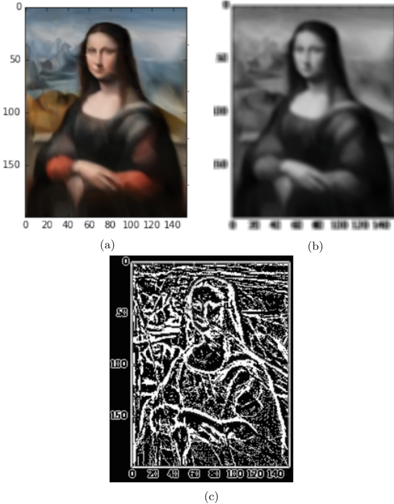
Fig. 3. (a) Original image. (b) Result of the convolution of the original image with a 3 \times 3 \times 3 kernel where all elements have 1/27 value. This kernel is a smoother. (c) Result of the convolution of image (b) with the kernel defined in Eq. (7). This kernel is an edge detector.
