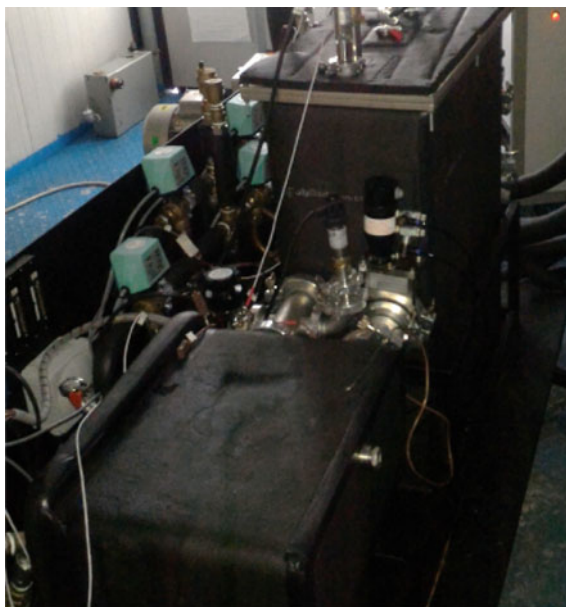
Fig. 4 The adsorption TES system developed at CNR-ITAE
