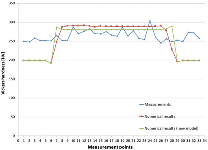
Fig. 10 Comparison of measured and calculated hardness distribution on 4th welded bead
