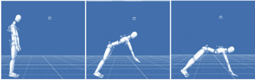
Fig. 4 Faller’s body configurations at different stages of the falling process obtained by the Opti-track system
