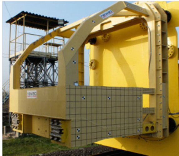
Fig. 3 Anti-climbing plates instead of side absorbers [7]
