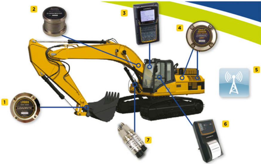
Fig. 1 Components of Load Rite X2350 system by Trimble [6]: 1—inclination sensor for determination of angular position of bucket, 2—inclination sensor for determination of angular position of boom, 3—control panel (HMI), 4—sensors for determination of ground inclination, 5—wireless data transmission device (wi-fi, GPRS, radio communication), 6—printer, 7—sensors for determination of oil pressure inside boom positioning hydraulic cylinder/cylinders
