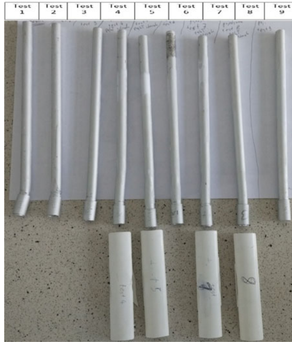
Fig. 9 View of aluminum tubes after tests on Charpy hammer with various angle of inclination and masses
