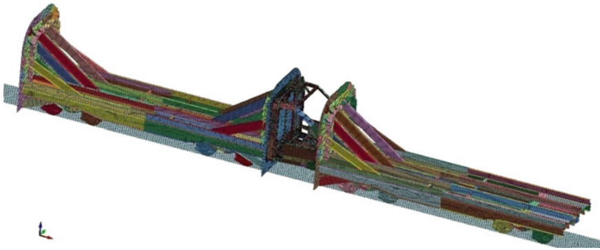
Fig. 8 Finite element mesh for the full model
