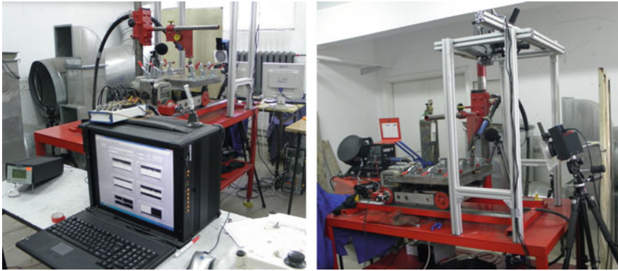
Fig. 1 Test stand with the computer station and the welding device
