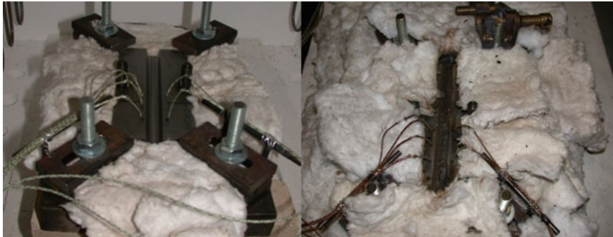
Fig. 2 View of 10GN2MFA steel specimen with thermocouples and Sibril isolation before heating (on the left side) and during welding (on the right side)
