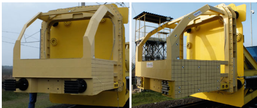
Fig. 1 Driver's cab with and without the side absorbers [7]
