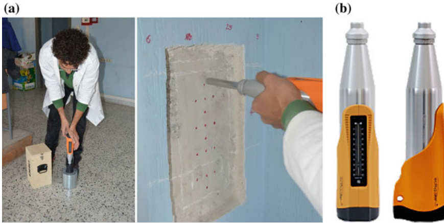
Fig. 4 a Calibration check e sclerometric test, b Ectha1000 DRC Sclerometer
