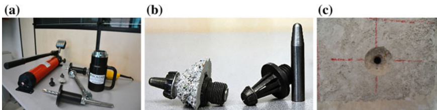
Fig. 5 a Pull-out test equipment, b BOVIAR Thoro dowel, c Surface rupture
