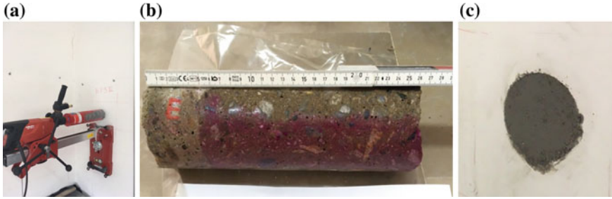
Fig. 6 a HILTI DD150-U diamond drilling systems, b Measurement of hardened concrete carbonation depth, c Hole sealing material
