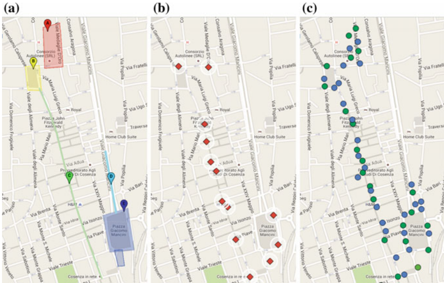
Fig. 2 Smart Street Cosenza. a Target areas; b Computational Nodes; c Sensors nodes. Green locations host one type A node and one type B node, blue locations hosts only a type A node
