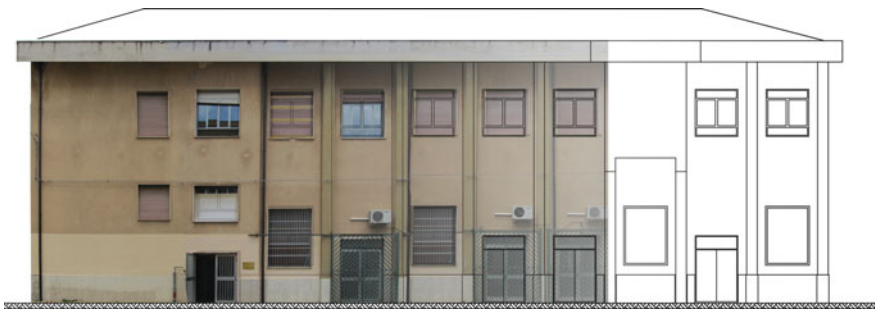
Fig. 3 Reconstruction of an elevation from orthogonalized images
