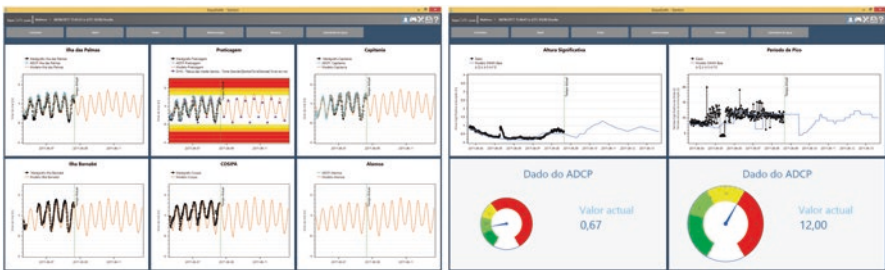
Fig. 7.14 Workspace showing the data measured by the six tide gauges and the model’s results for sea level (left). Workspace showing the results of the wave model and the measured data on significant height and peak period (right)
