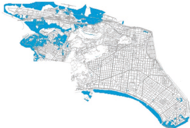
Fig. 7.20 Areas of the city of Santos (in blue) that are susceptible to flooding, given a tide of 2.48 m. (Source: Berzin and Ribeiro 2010)
