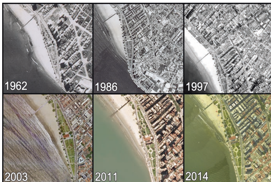
Fig. 15.3 Historical aerial imagery from 1962 to 2014 showing the progressive erosion at Ponta da Praia suburb. (Image kindly provided by the Prefecture of Santos)
