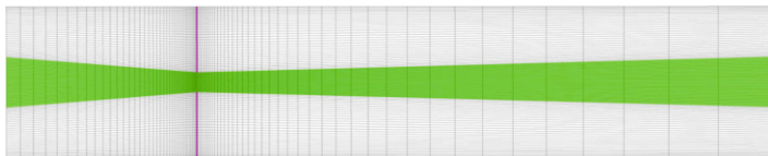
Fig. 9 The reference configuration of the body-fitted mesh for the 2D valve problem, with leaflets highlighted in magenta and areas of softened mesh highlighted in green
