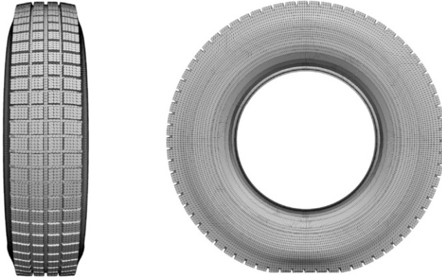
Fig. 17 Tire aerodynamics with an actual tire geometry. Deformed shape
