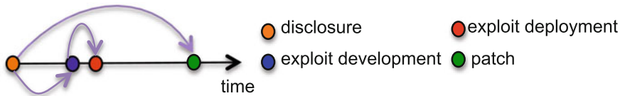
Fig. 8 Time dependencies between vulnerability lifecycle phases (purple arrows represent transitions between phases)
