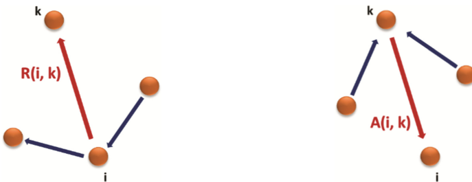
Fig. 4. Responsibility message R(i,k) from i to k Fig. 5. Availability message A(i,k) from k to i
