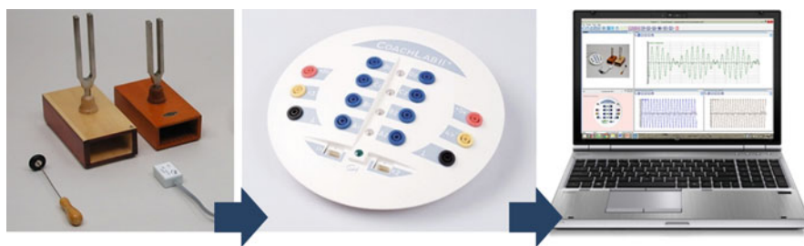
Fig. 3.1 Diagram of the tool for data logging with sensors (incl. sensor, interface, and computer with dedicated software)
