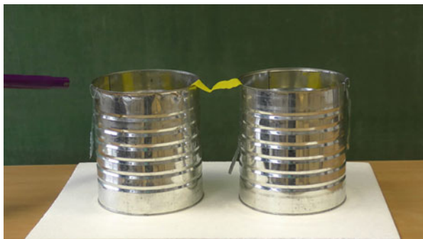
Fig. 6.8 Charge transport from a left tin to a right one (using a piece of crepe paper as a conductor)
