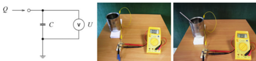
Fig. 6.7 Simple measurement of charge of a plastic straw
