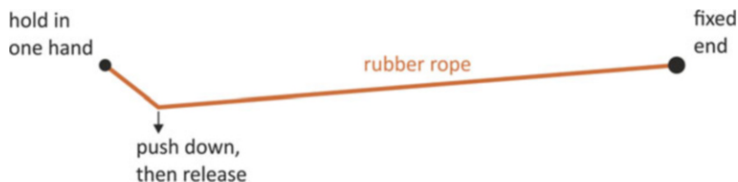
Fig. 6.11 How to demonstrate transversal travelling wave on a rubber rope
