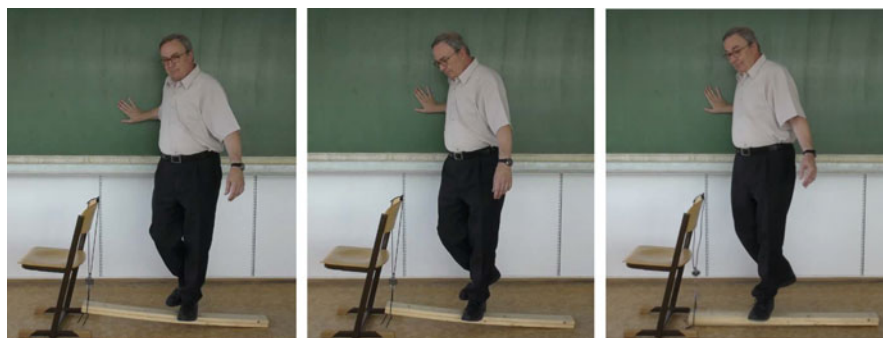
Fig. 6.15 A simple way how to measure (at least approximately) the force for pulling magnets apart: stepping at different points of the board changes the force
