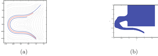
Fig. 1. (a) Simulation for Example 1 showing flowpipe segment being extremely stretched and deformed, (b) Interval over-approximation of the Taylor model computed by Flow* [3].
