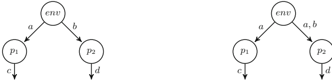
(a) An architecture of two processes that specify process p_1 to produce c from a and process p_2 to produce d from b . (b) The same architecture as on the left, where only the inputs of process p_2 are changed to a and b .
