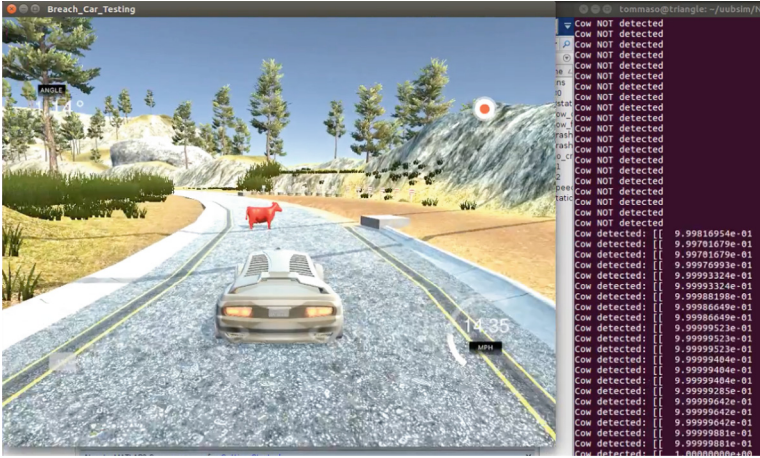
Fig. 6. Udacity simulator with a CNN-based AEBS in action.
