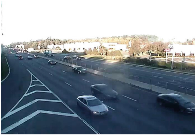
Fig. 1. A frame from a traffic video. The RGB values of some foreground regions, i.e., vehicles, are similar to the RGB values of the background, namely, the lanes of the road.
