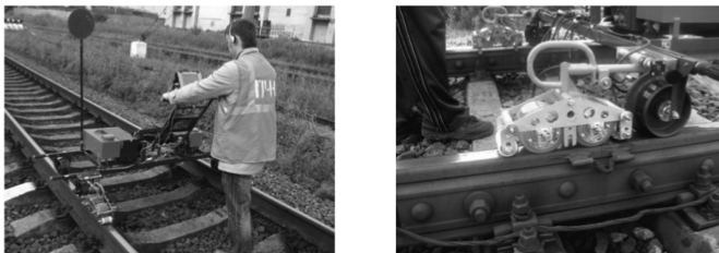
Fig. 1. The modern flaw detector AVICON-14
