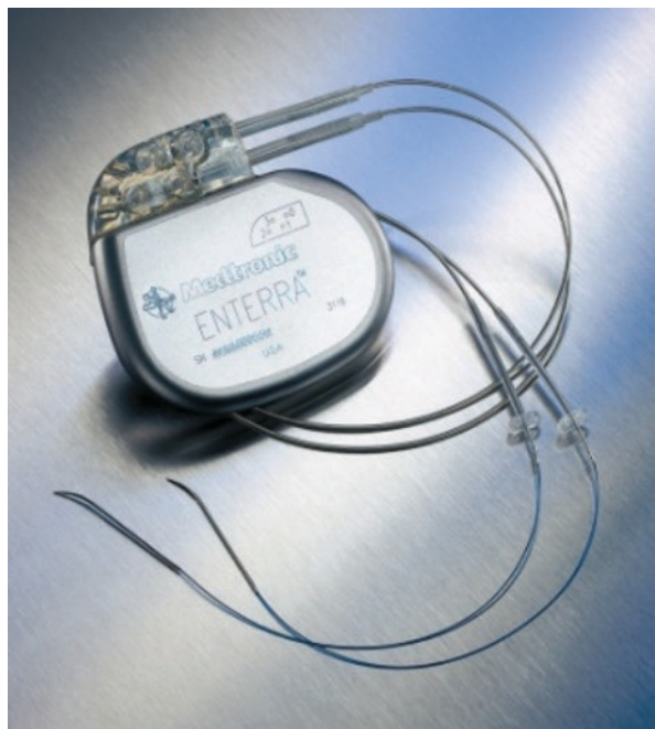
Fig. 72.1 Gastric electrical stimulator (GES) electrodes and pulse generator (Enterra, Medtronic, Minneapolis, MN, USA)
