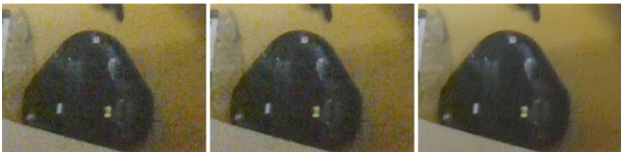
Fig. 7.10 Comparison of the application of the method proposed in [14] with a single scale or with three scales. From left to right: original noisy image, single-scale denoising, and three-scale denoising. The displayed denoised images have been enhanced [26] in order to better illustrate the differences between the two methods. The single-scale algorithm actually removes noise but only noisy regions of slightly more than one pixel, not large spots. Large colored spots are removed only by the multiscale algorithm, which removes them at the scale for which they become almost white noise
