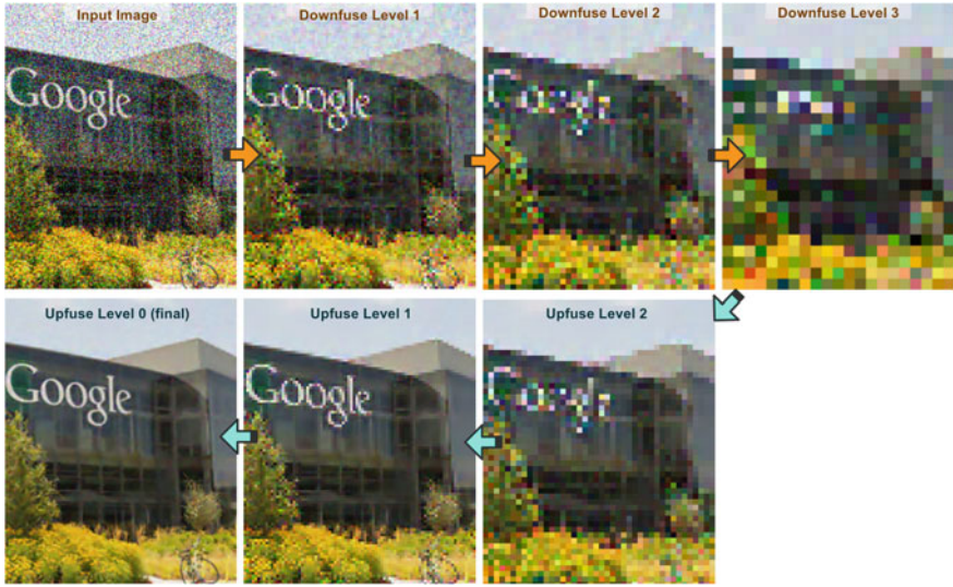
Fig. 10.2 This series of images shows the progression of NLM pull-push filtering of an image through the downfuse and upfuse stages. Notice how the noise is reduced throughout the stages
