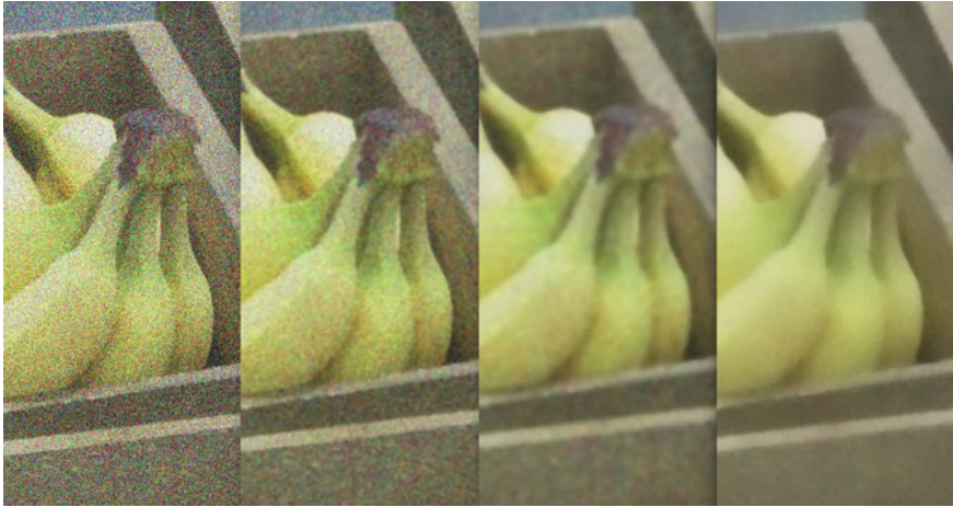
Fig. 10.7 From left to right, image with additive Gaussian noise with \sigma_n = 85 (SSIM:0.065), 7 \times 7 NLM (SSIM:0.799), 15 \times 15 NLM (SSIM:0.918), and pull-push NLM (SSIM:0.935)
