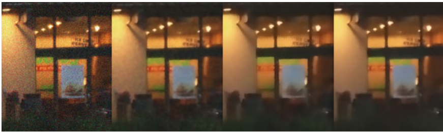
Fig. 10.8 From left to right, image with additive Gaussian noise with \sigma_n = 60 (SSIM:0.132), 7 \times 7 NLM (SSIM:0.873), 15 \times 15 NLM (SSIM:0.927), and pull-push NLM (SSIM:0.935)
