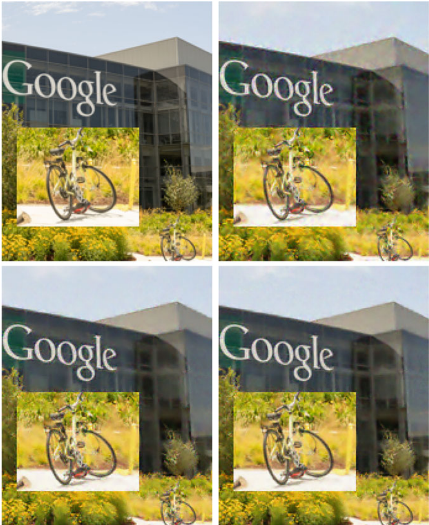
Fig. 10.13 Burst pull-push NLM: The upper left image shows the noiseless base frame of the nine frame burst from the previous figure. The upper right image shows the result of single frame pull-push NLM on this frame (SSIM:0.844). Using the simple approach to burst processing (lower left) provides better results (SSIM:0.868), but in highly textured regions is only able to incorporate nearby frames due to limited motion compensation. Using the motion compensated burst processing (lower right) allows for the best quality result (SSIM:0.900)
