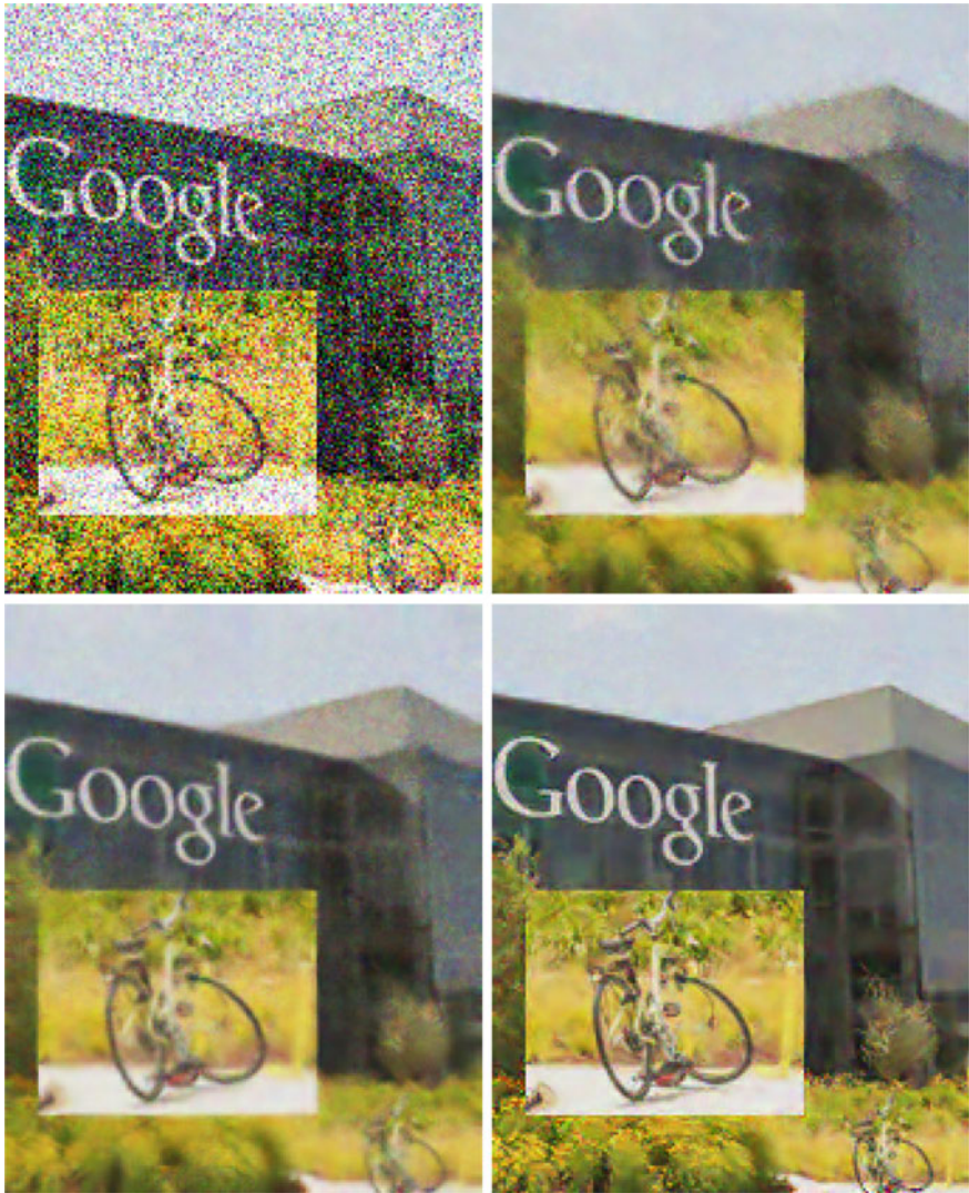
Fig. 10.16 This figure shows the results with much higher added synthetic noise level \sigma_n=60 . The first row shows, the noisy base frame (SSIM:0.239), and non-motion compensated pull-push burst NLM (SSIM:0.619). The second row shows motion compensated pull-push burst NLM (SSIM:0.675) and motion compensated joint burst pull-push NLM (SSIM:0.805)
