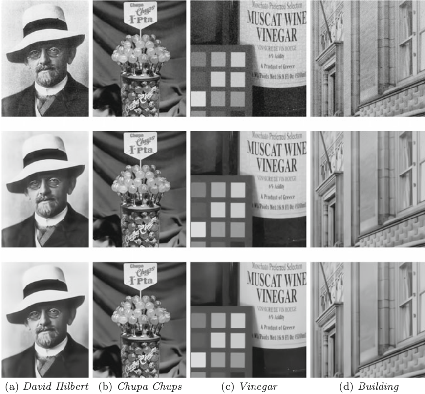
Fig. 4.9 Grayscale image denoising results by different methods on real noisy images. From top to bottom: noisy images, denoised images by BM3D, denoised images by FFDNet. a \sigma = 15 ; b \sigma = 10 ; c \sigma = 20 ; d \sigma = 20
