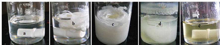
Fig. 22 The photographic image of transformation of casting solution during the preparation of polysulfone and chitosan blend membrane [97]. (Reproduced with permission of Royal society of chemistry)
