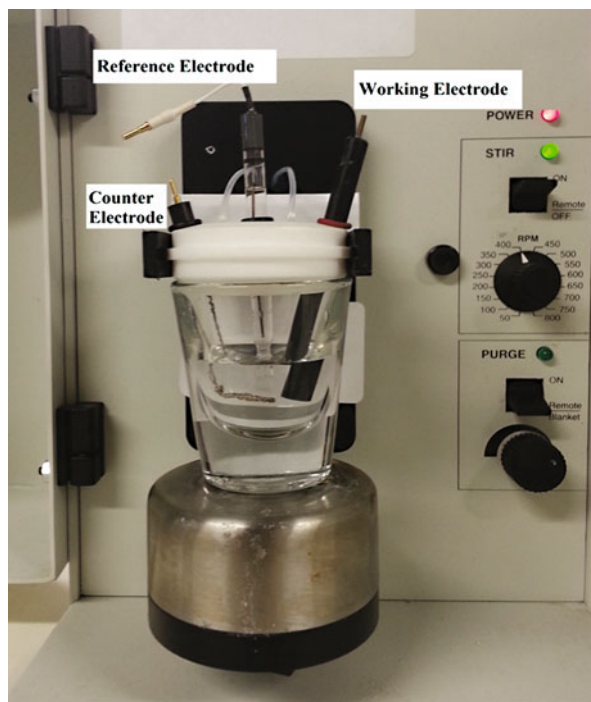
Fig. 10 Three-electrode setup for electrochemical synthesis of conducting polymers – reference electrode, working electrode, and counter electrode
