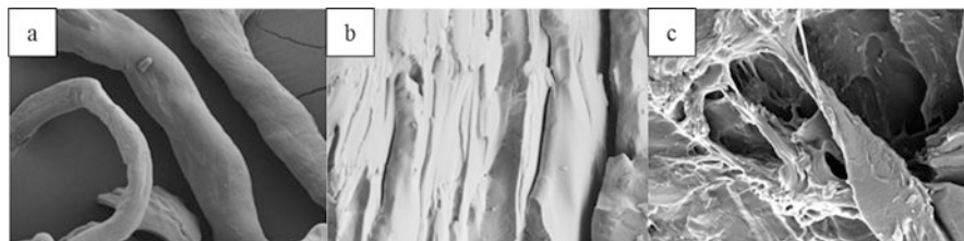
Fig. 13 FESEM of: (a) CMC, (b) PAM, (c) CMC-g-PAM [104]. (© The authors, ( https://www.sciencedirect.com/science/article/pii/S1110062114200109#! ), according terms of Creative Commons Attribution 4.0 International License ( http://creativecommons.org/licenses/by/4.0/ ))
