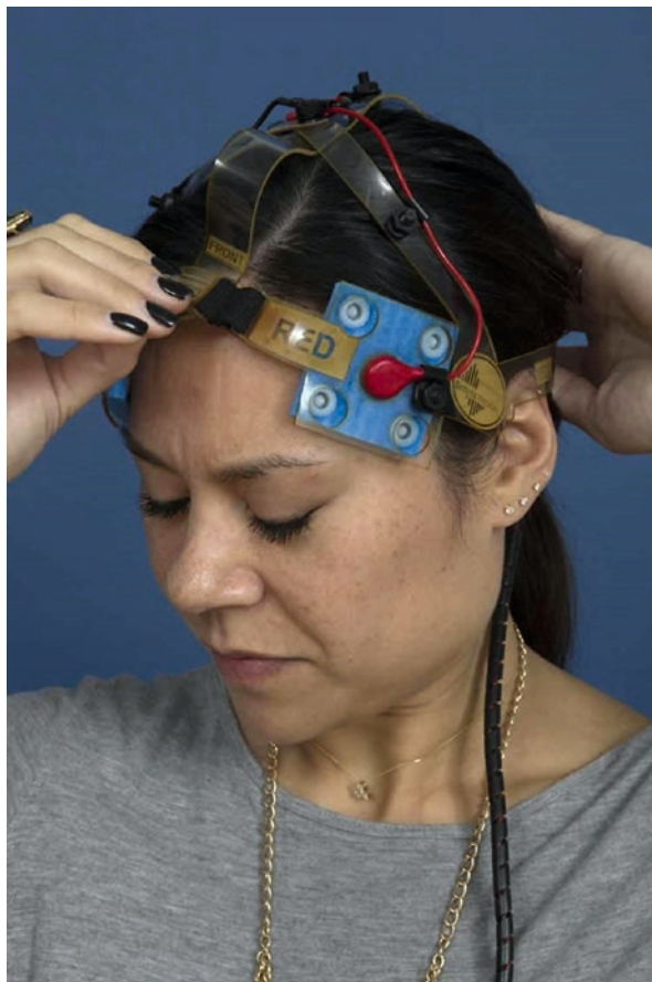
Fig. 13.1 4 × 4 tDCS headgear. Custom-made headgear has been modified with the goal of simplifying placement and minimizing dependence on manual dexterity. Electrodes will be securely attached to specific markings on the headset with the use of pre-moistened sponges. The sponges are provided in single-use packets, and once opened, can be readily attached in the correct placement to the headgear. A marker guides accurate user placement of the headgear. (The figure is courtesy of L. Charvet)
