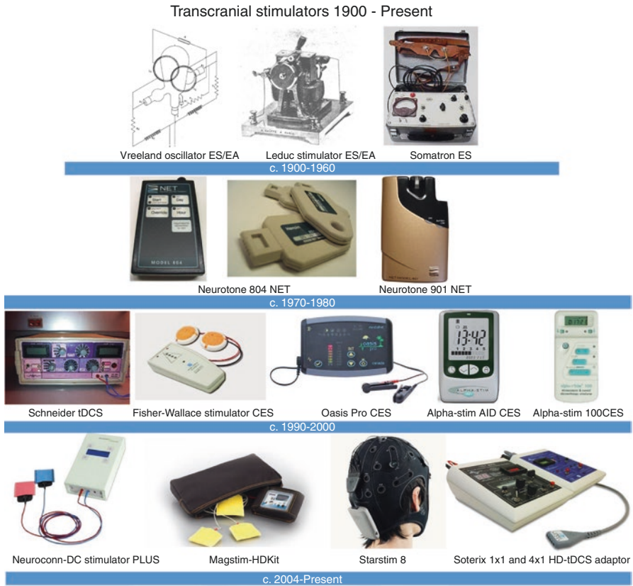
Fig. 1.3 The evolution of transcranial stimulators spanning 1900 to present day. Early ES/EA devices were developed between 1900 and 1960. These early devices were followed NeuroElectric Therapy (NET) devices between 1970 and 1980. Later more established tDCS, tACS, and iontophoresis devices were developed, some of which are still used today. During the early aughts, more advanced and modern stimulation techniques were developed starting from 2004 to present day
