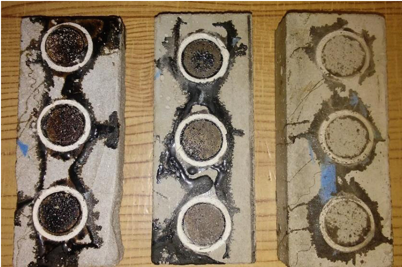
Fig. 6. Cement mortar substrate after pull-off test (left-Type A binder, middle-Type B binder, right-Type C binder)
