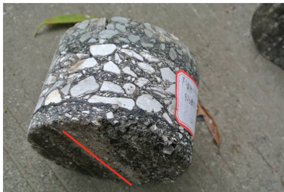
Fig. 6. The location of slab joint
