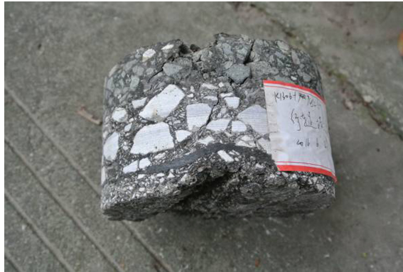
Fig. 7. The geotextile had moved upward
