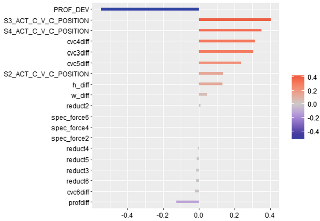
Fig. 7. The deviations of the model variables from the good products for a selected observation.
