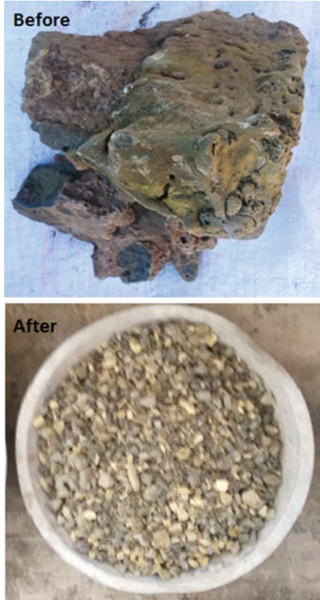
Fig. 1. The raw and graded rushed melted brick
