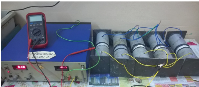
Fig. 3. Chloride ion penetration test setup
