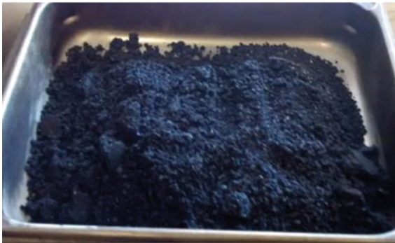
Fig. 2 7.5% asphalt content for crushed fine mixture
