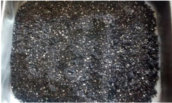
Fig. 1 5.5% asphalt content for crushed fine mixture
