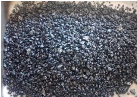
Fig. 3 2.5% asphalt content for 1/4" aggregate mixture
