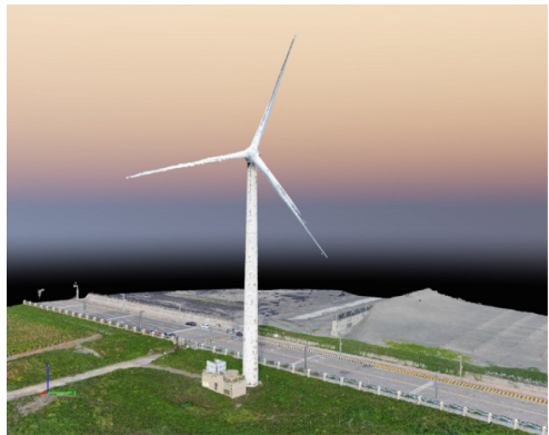
(b) The Point Cloud Generated from UAV
