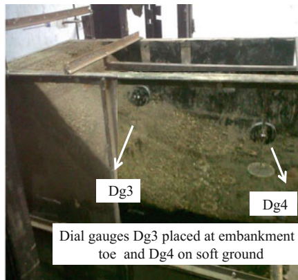
Fig. 2. Dial gauges placed at different location in the model tests: a Dg1 and Dg2 for vertical settlements; b Dg3 at embankment toe and Dg4 on soft foundation for heaving measurement
