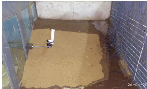
Fig. 21. Slope failure - 28° [soil - 2]
