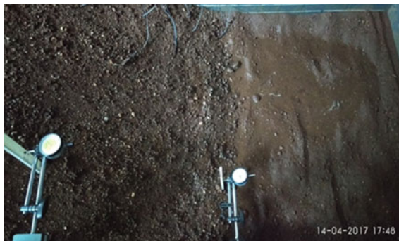
Fig. 15. Slope failure - 30° [soil - 1]
