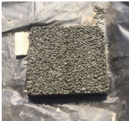
Fig. 5. Slab after removing the formwork
