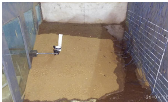
Fig. 21. Slope failure - 28° [soil - 2]
