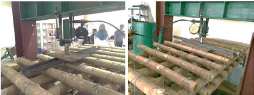
Fig. 7. Loading tests on bamboo mattress.
