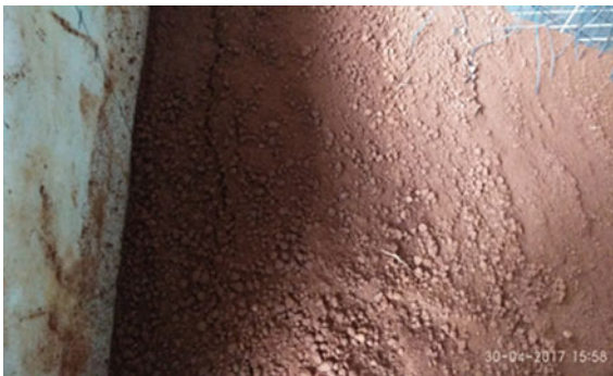
Fig. 27. Slope failure - 30° [soil - 3]
