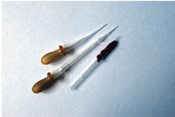
Fig. 14.2 Some handmade preparatory aids: micropipettes made from eye dropper and commercial micropipette tips and adjusted entomological pin
