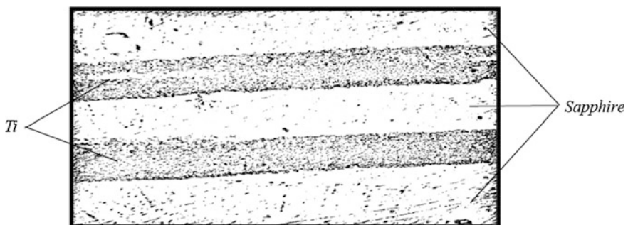
Fig. 3 Fractographic picture of the sapphire surface with titanium after destruction of the joint ( T = 850 \text{ }^\circ\text{C} ; P = 14.7 \text{ MPa} , t = 7 \text{ min} , \times 450 )
