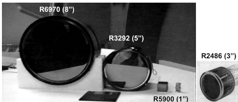
Fig. 6.12 Hamamatsu PSPMT models belonging to first and second generations (reproduced from: Pani R, Pellegrini R, Soluri A, De Vincentis G, Scafè R, Pergola A. Single photon emission PMT. Nucl Instr & Meth A 1998;409:524-8, Figure 2)
