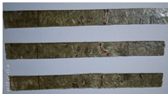
Fig. 3.4 Tensile test specimen of jute fiber reinforced composite
