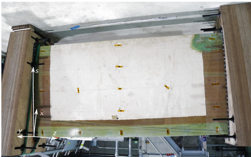
Fig. 33.5 Specimen coordinate system in suction side view. Root end is on the left and tip end on the right hand side
