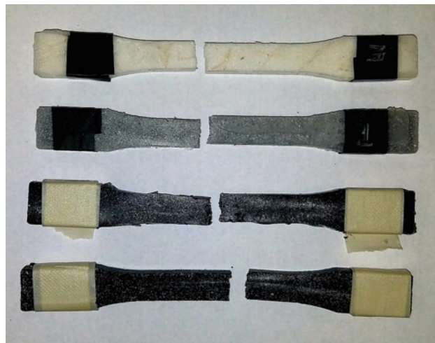
Fig. 21.4 Image of tension specimen for each material system – post failure. From top to bottom: Sugar PDMS, Sugar Aluminum PDMS, Sugar CNT PDMS, Sugar Aluminum CNT PDMS
