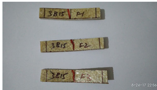
Fig. 3.5 Flexure test specimen of banana fiber reinforced composite
