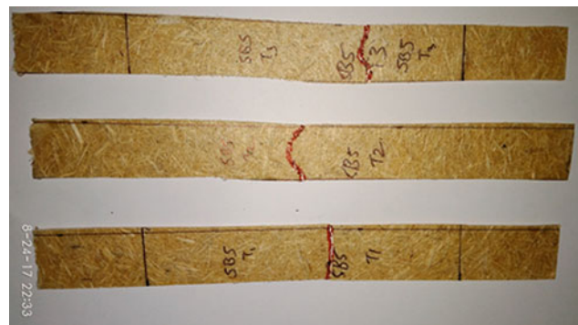
Fig. 3.3 Tensile test specimen of banana fiber reinforced composite
