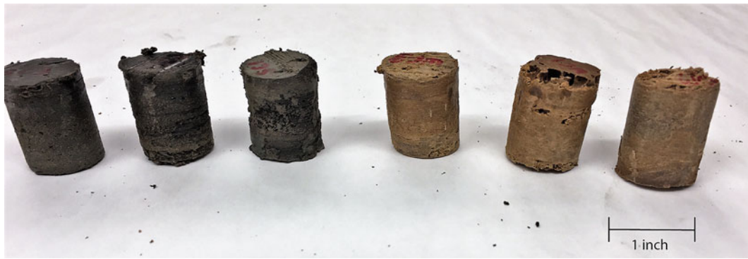
Fig. 32.2 Cylindrical samples for compression tests
