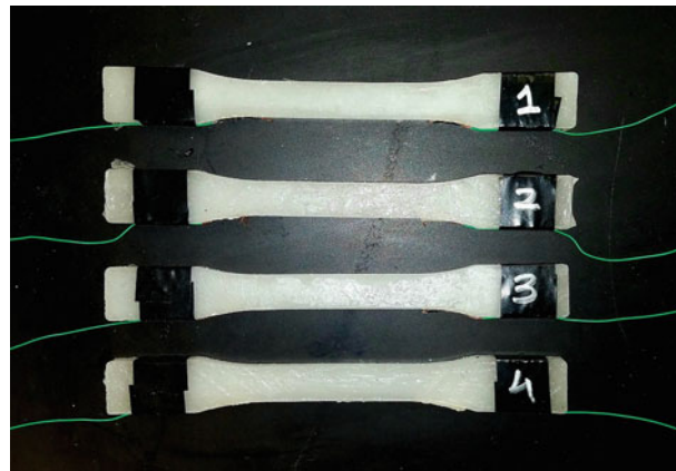
Fig. 21.2 Image of tension Neat Sugar PDMS specimen with side electrode placement
