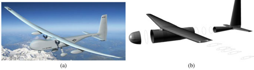
Fig. 30.12 Representation of (a) the Orion UAV designed by Aurora Flight Sciences and (b) the parametric NURBS based model used for IGA simulations
