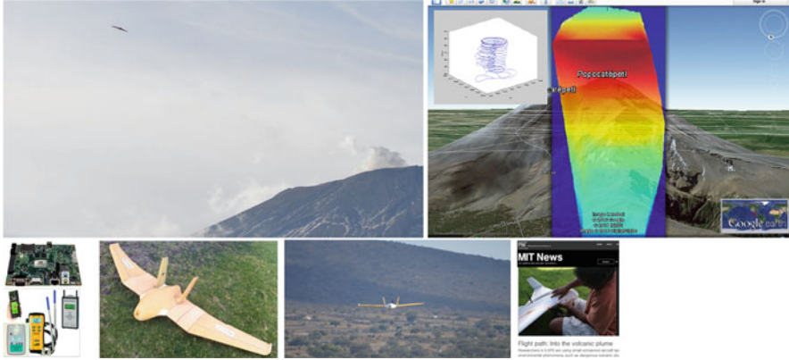
Fig. 2.1 MIT Cooperative Autonomous Observing System at the Popocatepetl Volcano in an experiment to gather and produce SO_2 maps using sUAS for in-situ and remote sensing. Shown here is an aircraft in flight, flight path and inversion for concentration, typical sensors, the aircraft and press coverage
