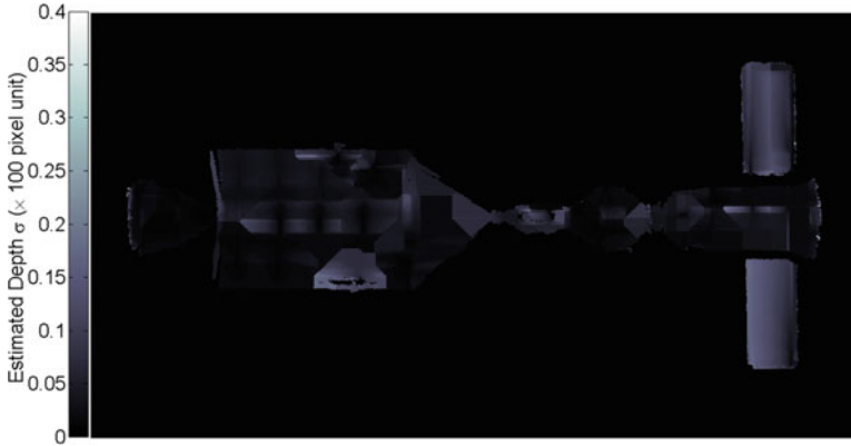
Fig. 13.34 Estimate surface depth standard deviation map of spacecraft model with specular reflection
