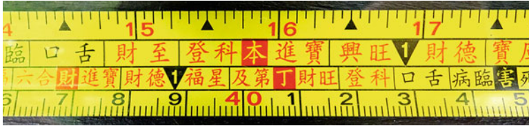
Fig. 3.14 Modern metal Luban measure, combining the measure for good yin and yang fengshui. Yang is arranged at the top, yin at the bottom of this measure
