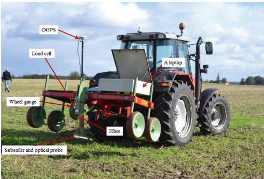
Fig. 3 The on-line visible and near infrared (vis-NIR) soil sensor [25]
