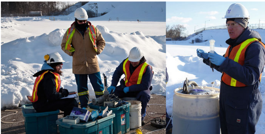
Fig. 7.7 Sampling on a NZVI test site (left) and on-site screening and sample preservation for laboratory analysis (right)
