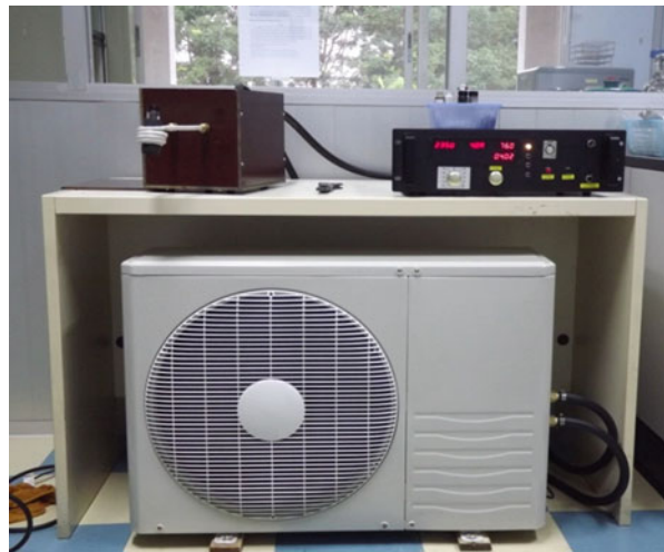
Fig. 11.5 EMF generator and an induction coil (white coil) to hold vials for induction heating and LF EMF-enhanced dechlorination experiments
