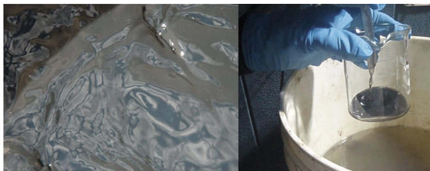
Fig. 7.9 NZVI slurry synthesized at 1 g/L in 0.8% wt CMC prior to injection (left). NZVI sample collection at a monitoring well downstream of the injection (right)
