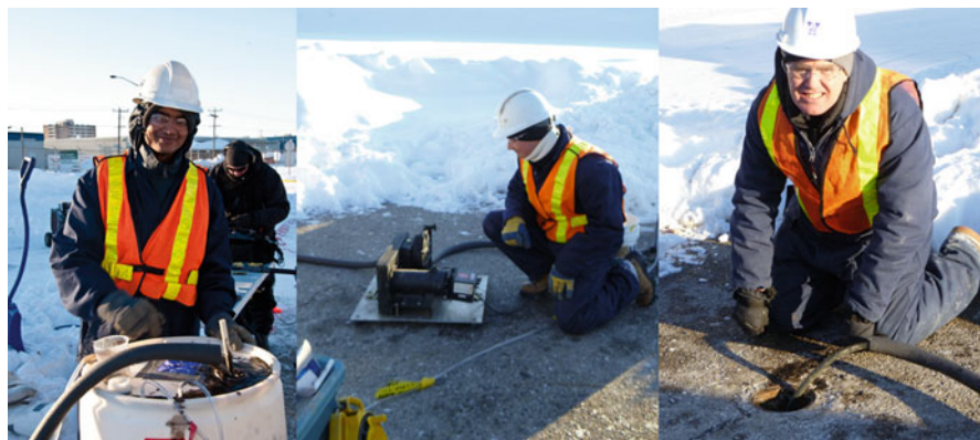
Fig. 2.1 NZVI slurry ready for injection. (Photo with permission from Kocur, Sleep and O'Carroll)
