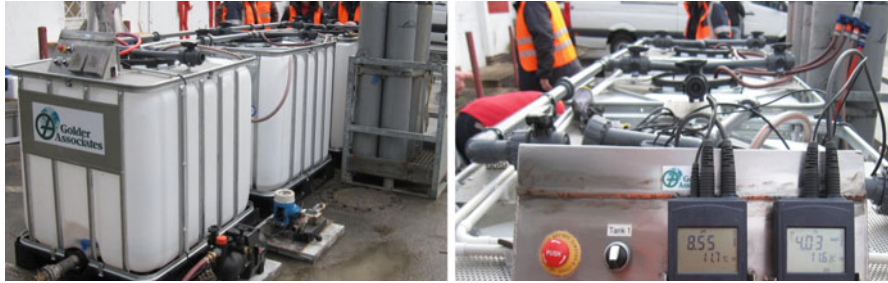
Fig. 8.7 Example of slurry field mixing and injection equipment (Doose and Bruns 2014). The NZVI slurry is a mixture of water with NZVI particles typically up to 10–20 g/L of NZVI powder mixed with surface modifiers to maintain NZVI particles in suspension and prevent NZVI agglomeration, and additional catalysts (e.g. palladium acetate) to accelerate contaminant reduction or to reduce recalcitrant constituents
