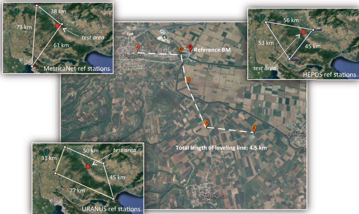
Fig. 1 Maps showing the location of the test points (A–E), the reference benchmark of the national vertical datum, and the nearby permanent stations of the three GNSS/NRTK positioning networks
