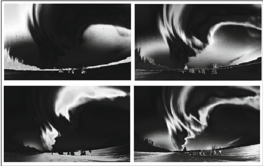
Fig. 3. Classes applying fuzzy 4-means algorithm (top left: class 1, top right: class 2, bottom left: class 3, bottom right: class 4) The gray scale represents the membership degree of each pixel to each class, where black = 0 and white = 1
