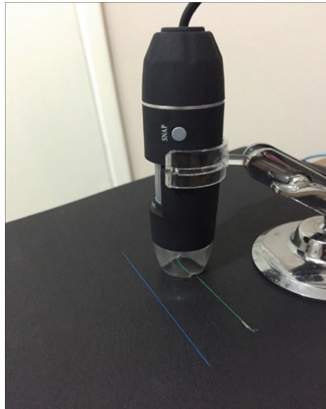
Fig. 2. Experimental setup: USB camera and optical fibers.
