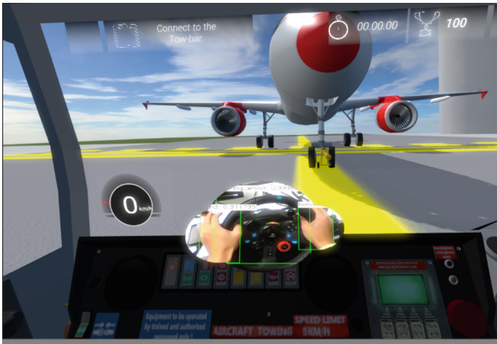
Fig. 7. User's perspective while controlling the tow truck. The driving wheel and driver's hands are detected and blended into the virtual environment.
