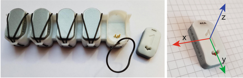
Fig. 1. Photos of the PostureSensei TM sensor system. Four of five sensors are sitting in the charger. A single sensor has the dimensions 33 mm × 16 mm × 10 mm and is attached to a person's back with double sided tape. The right images shows a sensor's local coordinate system.
