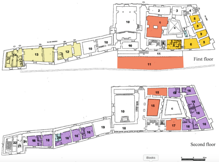
Fig. 5. Layout scenario 3. Legend: c. cloister; 1. restaurant 30 places; 2. reception; 3. services; 4. atrium; 5. kitchen stores; 6. kitchen; 7. bathroom; 8. kitchen extension; 9. elevator; 10. premises of ecclesiastical property; 11. gallery, terrace and gazebo; 12. additional first level services and wellness center locker rooms; 13. wellness center; 14. wellness center locker rooms; 15. meeting room; 16. rooms; 17. breakfast room and bar; 18. wide corridor; 19. filter room; 20. common bathrooms; 21. deposits; 22. filter zone to the stairs and lift
