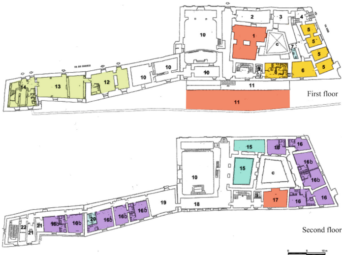
Fig. 3. Layout scenario 2. Legend: c. cloister; 1. restaurant 30 places; 2. reception; 3. services; 4. atrium; 5. kitchen stores; 6. kitchen; 7. bathroom; 8. kitchen extension; 9. elevator; 10. premises of ecclesiastical property; 11. gallery, ramp and terrace and gazebo; 12. additional first level services and wellness center locker rooms; 13. wellness center; 14. wellness center locker rooms; 15. meeting room; 16. rooms; 16b. loft rooms; 17. breakfast room and bar; 18. wide corridor; 19. filter room; 20. common bathrooms; 21. deposits; 22. filter zone to the stairs and lift.
