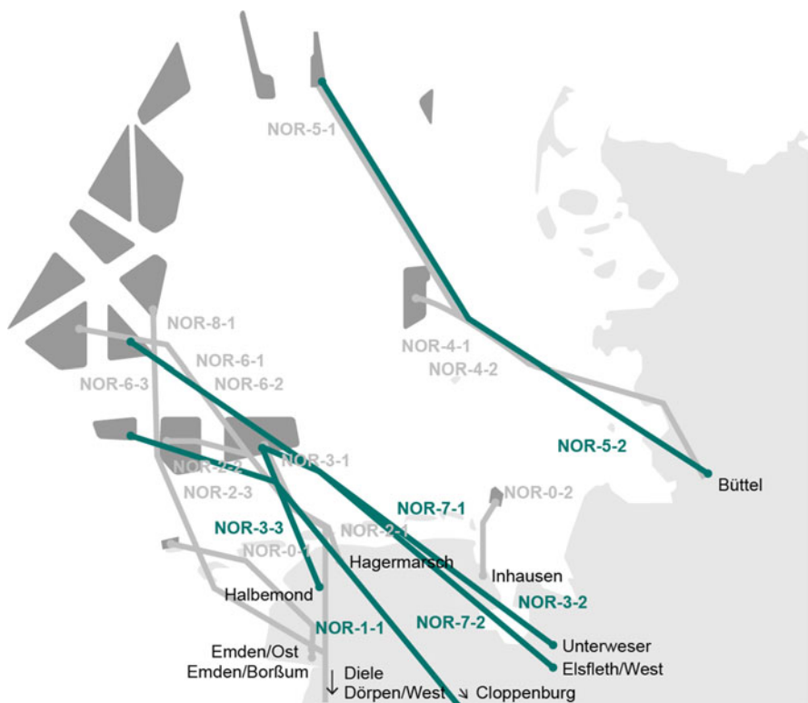
Fig. 8.2 Offshore Network Development Plan (NEP) for the German North Sea. The starting grid is gray; the projects of the scenario 2023B are in green. Source: Gerbaulet et al. (2013) (Gerbaulet, Clemens, Friedrich Kunz, Christian von Hirschhausen, and Alexander Zerrahn. 2013. “Netzsituation in Deutschland bleibt stabil.” DIW Wochenbericht 80 (20): 3–12)
