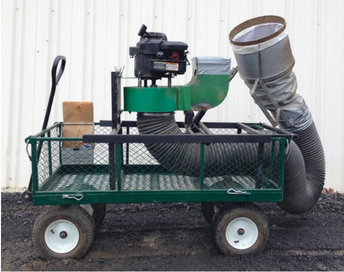
Fig. 11.2 Modified “D-Vac” for use in harvesting small plots of Asteraceae, Onagraceae, or other species seed with a pappus or fluff. Seed is vacuumed into a fine screen “sock” at the end of the flexible harvest hose. The sock and hose are cleaned between plots, so there is no cross-plot contamination
