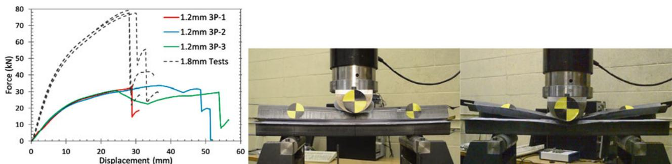
**Fig. 18.1** Force displacement of three point bend tests (left), with examples of symmetric failure (center) and asymmetric failure (right)
