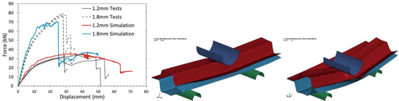
**Fig. 18.3** Comparison of experimental and numerical force-displacement plots (left) and predicted separation of flange (1.8 mm center, 1.2 mm right)
