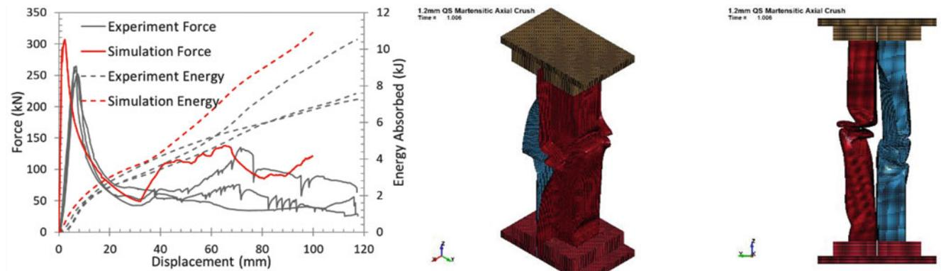
**Fig. 18.4** Comparison of experimental and numerical force-displacement plots (left) and predicted global buckling deformation mode (center, right)
