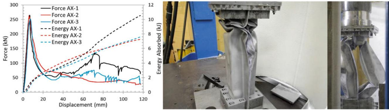
**Fig. 18.2** Force displacement of axial crush tests (left), with examples of local folding mode (center) and global buckling mode (right)
