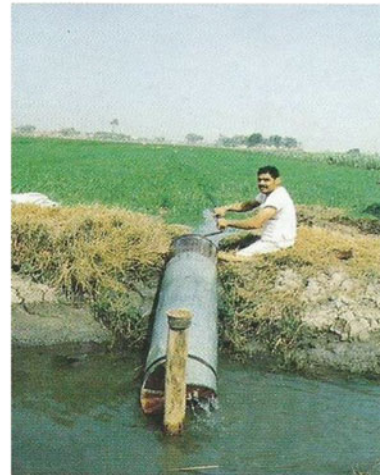
Fig. 5 (a) Lifting devices: the shadouf [8]. (b, c) Lifting devices: (b) the tambour (Archimedean screw) [9], (c) the sakia (waterwheel) [8]
