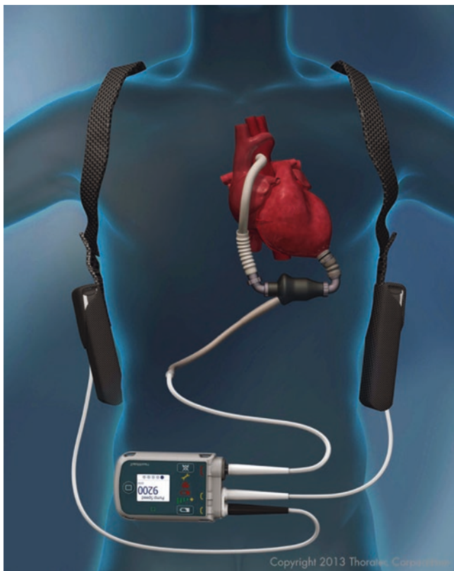
Fig. 18.3 HeartMate II LVAD implant orientation and patient peripherals. Percutaneous driveline exits the body and connects to device controller and power source. Battery power source illustrated here. (Courtesy Thoratec/Abbott)
