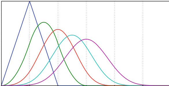
Fig. 1.3 The cardinal B-splines M_p for p = 1, \dots, 5 . The uniform knot positions are visualized by vertical dotted lines
