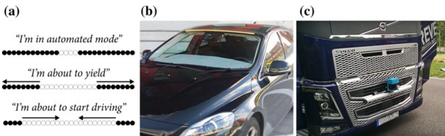
Fig. 2 The AVIP interface is dynamic (a). In passenger vehicles, it is placed on the top of the windshield (b); in trucks, it is placed in the middle of the grille (c)
