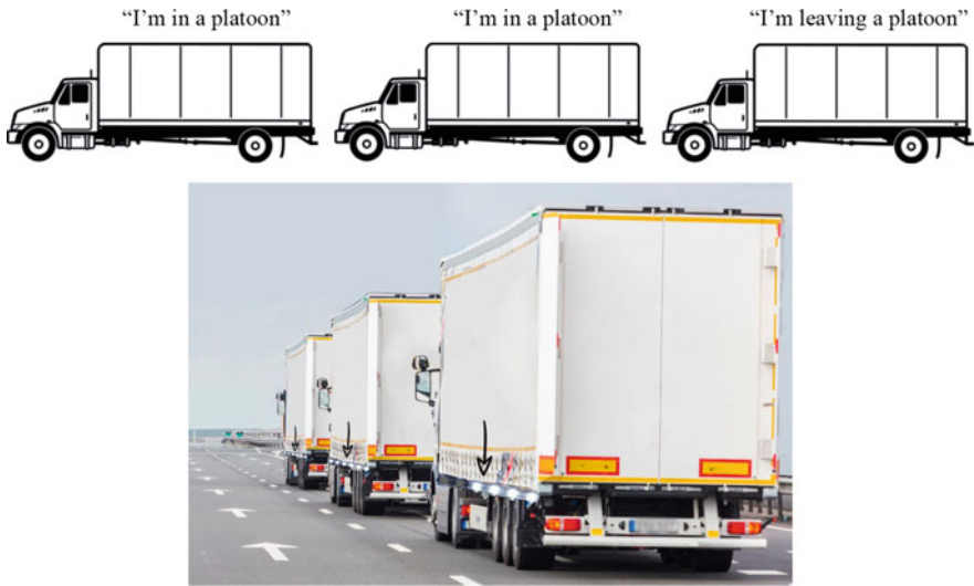
Fig. 3 The AVIP concept of communicating intent in the platooning scenario
